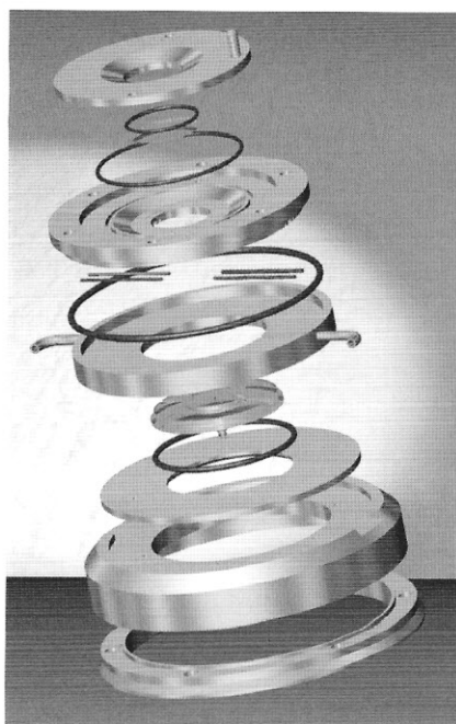
Figure 3: Blow-out diagram of the CFA flow chamber with its numerous stainless steel and rubber components, as well as the plexiglass central portion through which the solution to be analysed is perfused. Flow chamber dimensions are as follows: radius of the stagnation plate=1.1 mm, height (h) of the flow chamber=0.6 mm, radius of the inflow tube=0.3 mm.
