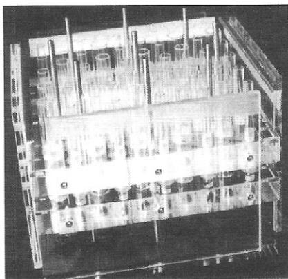
Figure 1: The filter block (a multi-channel filter device) consists of 50 incubation tubes inserted in a cube-shaped plexiglass frame construction. Each of the 10 rows has 5 incubation tubes with different volumes for simultaneous incubation with 5 different gas quantities. The bottoms of the tubes are closed by a rubber gasket pressed to the tube openings by a thick, screw-fixed plexiglass plate.
