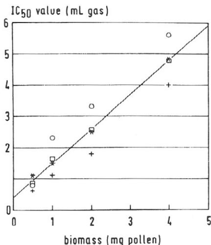
Figure 3: Linear correlation between  $IC_{50}$  values (mean inhibitory gas quantities) and biomasses (amounts of pollen in mg per ml culture medium) used in the experiment. Gas phase was taken from 3 different test cigarettes (o = type I, \* = type II, + = type III, □ = mean).
